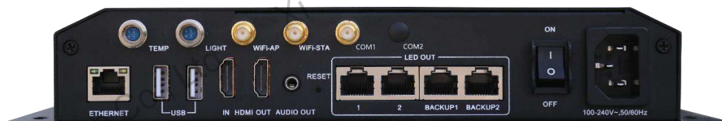
Figure 4-2 Rear panel of the TB6
